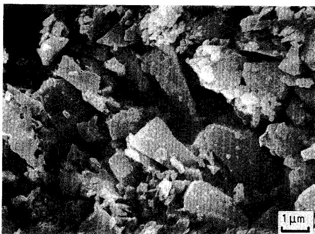
Figure 5 Microstructure of a mixture of HPZ amorphous silicon nitride with 5 wt % Y_2O_3 and 3 wt % Al_2O_3 fired to 1663 K. SEM micrograph corresponds to point A in Fig. 3.
